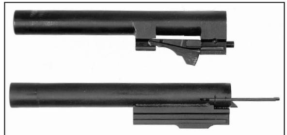
Lock up of the Ciener unit is different from that of the Beretta barrel as the tilting block is omitted. In its place is a large, single lug welded to the bottom of the barrel locked in place by the take-down latch.
